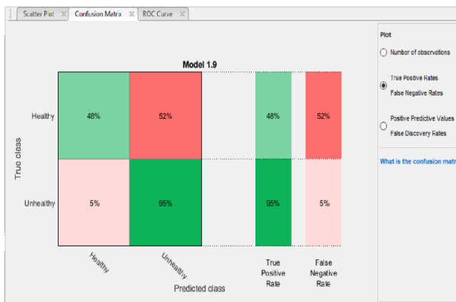
Fig. 14. Health classification model (Cubic SVM) confusion matrix of true positive and false negative rates.
