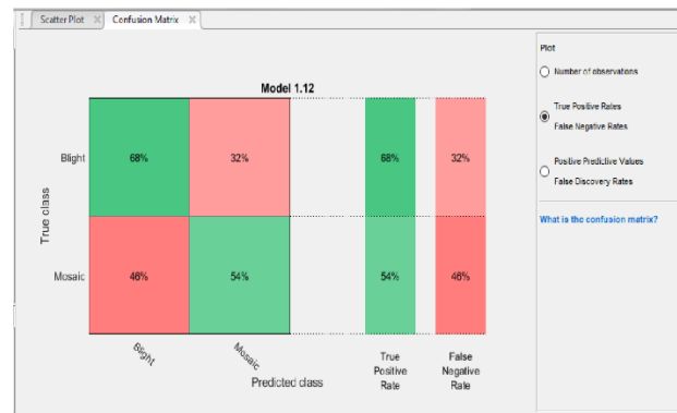
Fig. 21. Disease Classification Model of Confusion Matrix for True Positive and False Negative Rates
