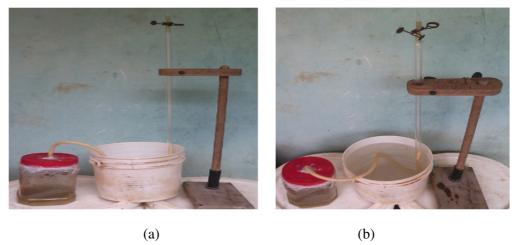
Figure 2.1: The picture of the fabricated biogas digester. (a) Side view of the set up. (b) The setup viewed from a steep angle of depression.
