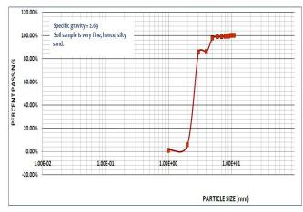
Fig 1.0: Particle Size Distribution Curve
