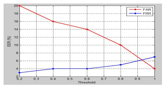
Fig. 2. Graph showing equal error rate for K-PCA
