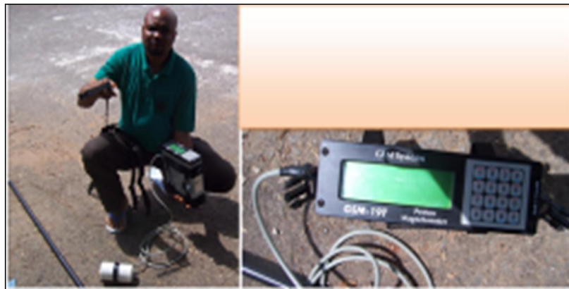
Fig. 2a. Portable magnetometer for ground magnetic survey
