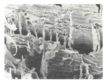
Figure 7. - Micrograph of a radial-longitudinal fracture plane in sound wood. The fibers (f) generally failed at steep angles (arrow) close to the S2 microfibrillar orientation. The ray/fiber interface (R) appears to be a weak plane where intercellular fractures occurred. Micrograph was taken from Type 1 fracture plane of a tension specimen.
