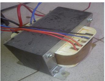
Fig.1. shell type transformer
