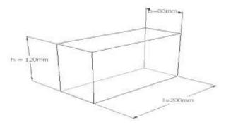
Figure 6 Isometric view of the Cutting chamber
