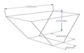
Figure 3 Isometric view of Exaggerated Hopper
