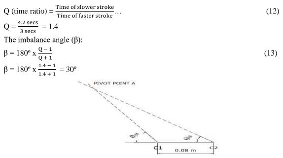
Figure 8 How to locate the axis of the pin joint C
