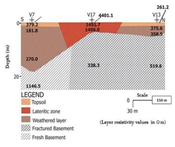
Fig. 10e Geoelectric section along profile 5.
