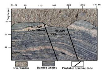
Fig. 7g Geomagnetic section of traverse 7.
