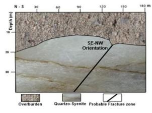
Fig. 7c Geomagnetic section of traverse 3.
