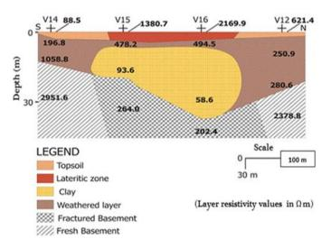
Fig. 10c Geoelectric section along profile 3.
