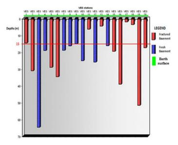
Fig. 11 Geoelectric evaluation of overburden thickness and basement nature.
