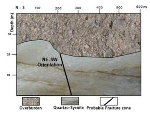
Fig. 7a Geomagnetic section of traverse 1.
