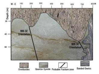
Fig. 7h Geomagnetic section of traverse 8.
