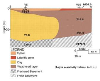
Fig. 10d Geoelectric section along profile 4.
