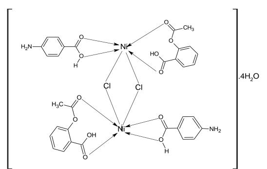
Figure 2: Proposed structure for the Ni(II) complex
